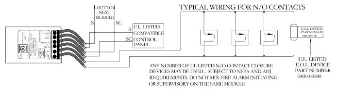
ALL CIRCUIT ARE SUPERVISED AND INHERENTLY POWER LIMITED
