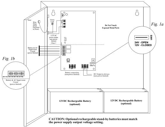
Keep power-limited wiring separate from non power-limited. Use minimum 0.25" spacing.
